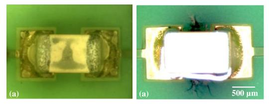
Figure 1: (a) Corrosion on the SMCs (after exposure to high humidity), and (b) corrosion under the SMC (after exposure to humid conditions, corrosion is induced by reflow flux residues)
