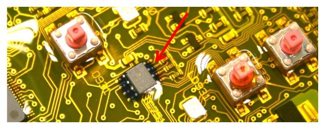
Figure 2: Reflow flux residue induced corrosion
