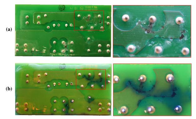
Figure 4: Tin corrosion under AC voltage (PCBA from the filed return): (a) before and (b) after application of the gel
