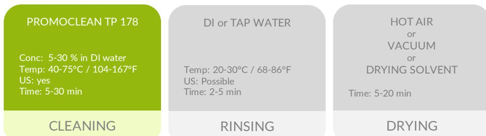
Diamond polishing compound removal (e.g. manufacturing of tungsten carbide cutting tools)
